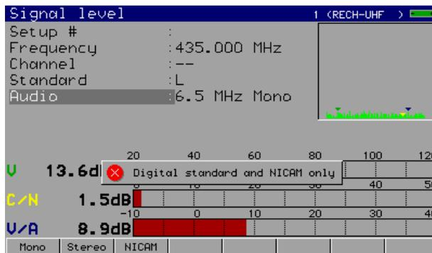
2<sup>nd</sup> press on the level key : The appliance tries to perform an error rate measurement with a **Standard** different from **DVB-C, MCNS, DVB-S, DSS, DVB-S2, DVB-T or NICAM**.
