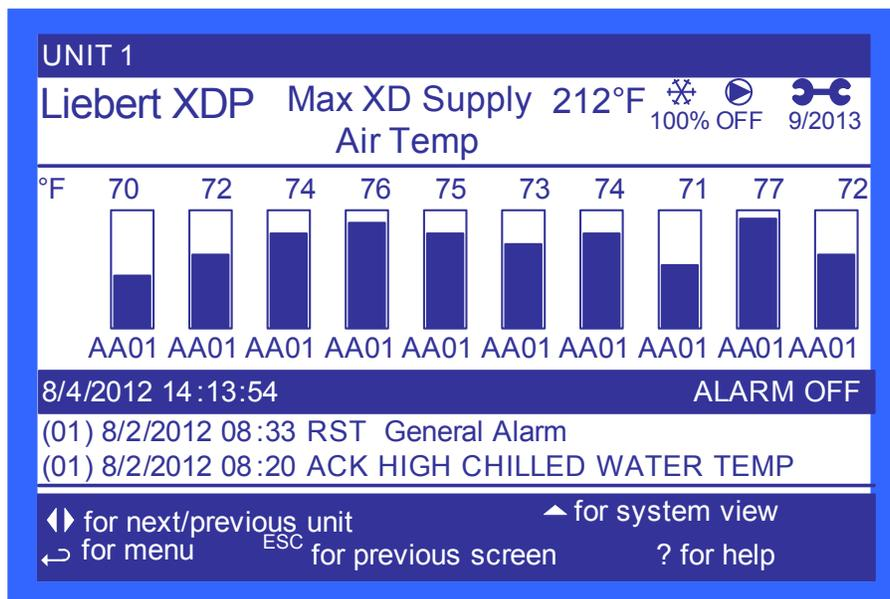
2. Press the down arrow button again to display the next 10 modules' outlet temperature and capacity levels.
