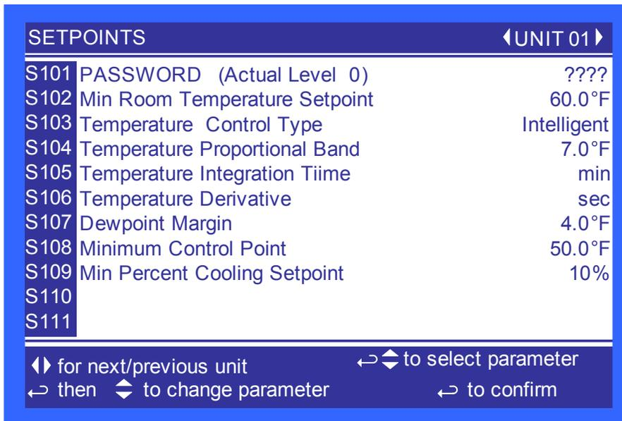
**Min Room Temperature Setpoint**—Sets the minimum room temperature the unit will attempt to maintain. If the temperature falls below this point, unit will raise the refrigerant temperature to reduce the amount of cooling. Adjustable from 50 to 80°F (10.0 to 26.7°C), the factory default setting is 60°F (15.6°C).
