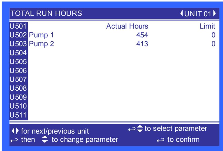
The parameter shows the actual hours Pump 1 and Pump 2 have operated and the maximum time Pump 1 can operate before the next maintenance.
