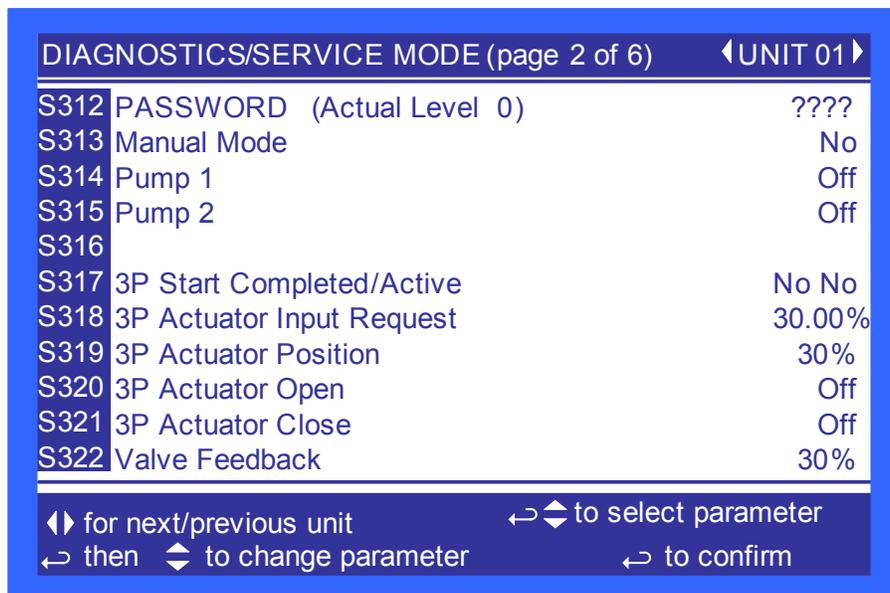
**Manual Mode**—Used to place the Liebert iCOM® control in manual mode. This is the initial setting necessary to activate any of the following items. When the Liebert iCOM is not in manual mode, each service menu item shows the current status of each parameter.
