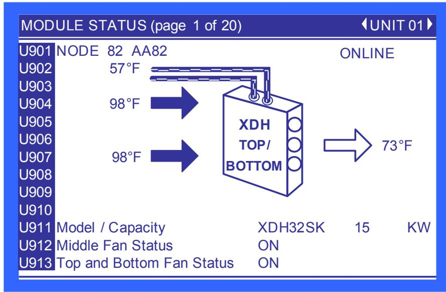
**U904**—Displays the temperature of the air entering the top of the bank of the Liebert XDH.
