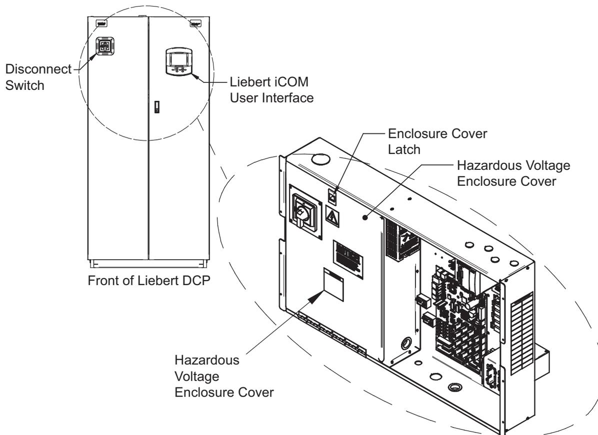
2. Determine which knockouts in the electrical enclosure will be used and remove them (see **Figure 10**).
