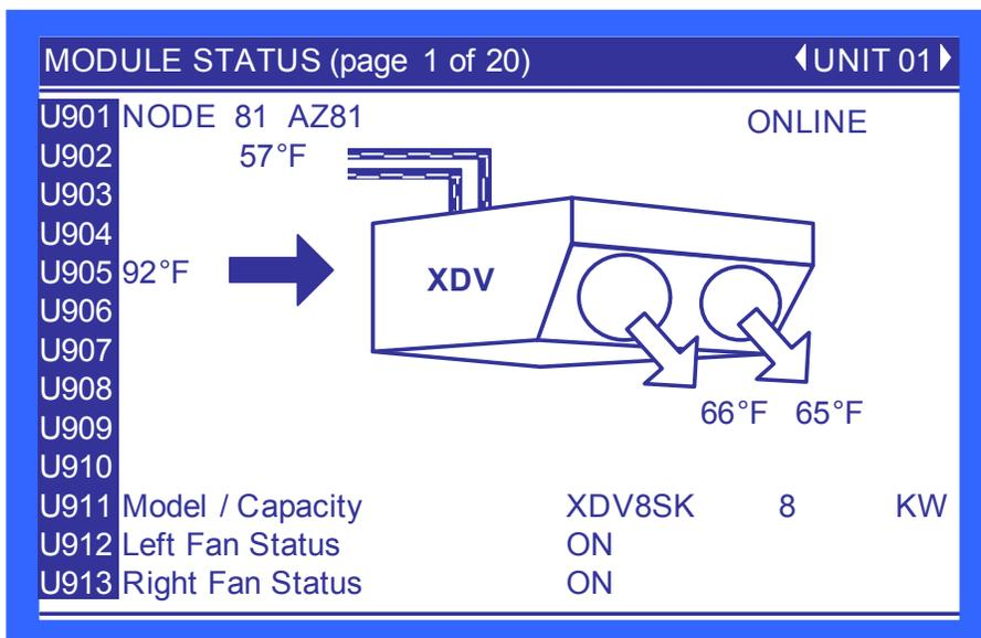
**Module Node ID**—The location within the CANbus. Each module's ID is factory-set to 80 and is automatically changed during setup; requires no user action.
