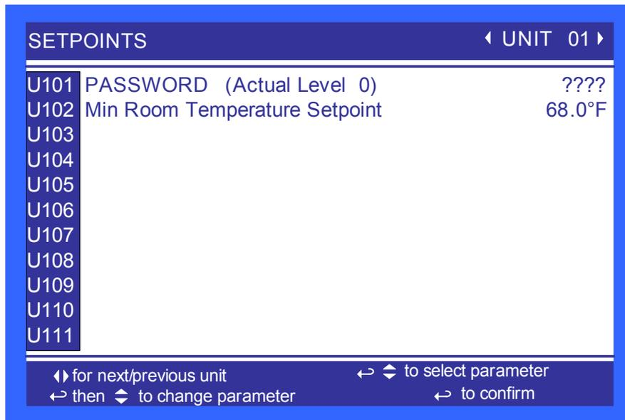
**Min Room Temperature Setpoint**—Sets the minimum room temperature the unit will attempt to maintain. If the temperature falls below this point, the unit will raise the refrigerant temperature to reduce the amount of cooling.
