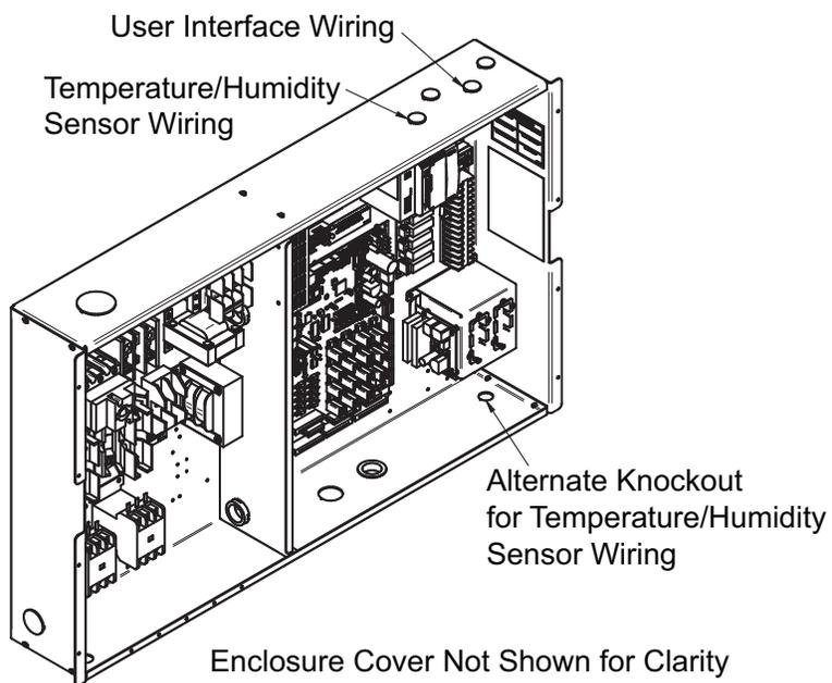
Figure 14 Connecting the remote temperature/humidity sensors
