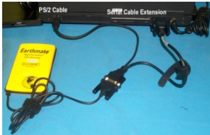
Figure 28 Setting up the GPS
