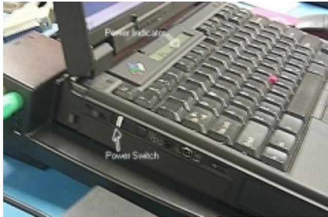
*Figure 2 Power Switch and Indicator*
