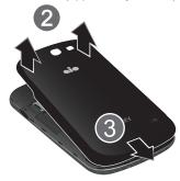
**Caution!** Do not bend or twist the back cover excessively.
