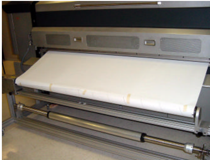
Figure 3-19 Attaching Media to the EMTU Core
