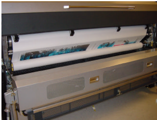
Figure 3-12 Rotate the Take-up Core
