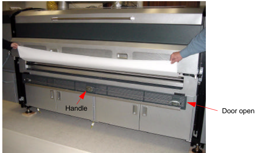
Figure 3-16 Open Paper-feed Access Door
