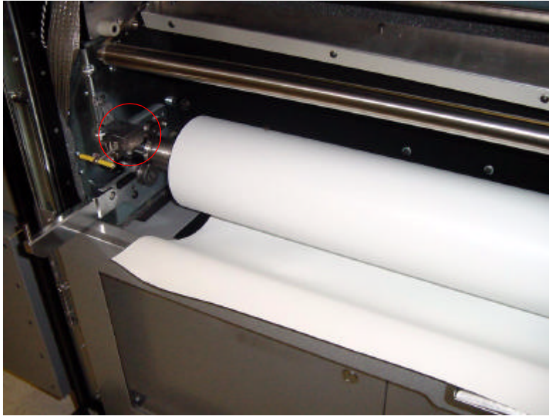
Figure 3-6 Secure the Mandrel/Media Assembly
