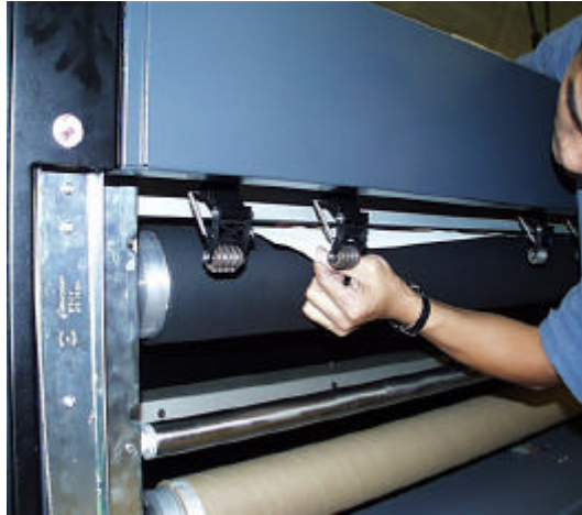
Figure 3-9 Feeding Media Over the Drive Roll
