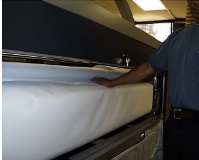
Figure 3-7 Feeding Media Over the Platen
