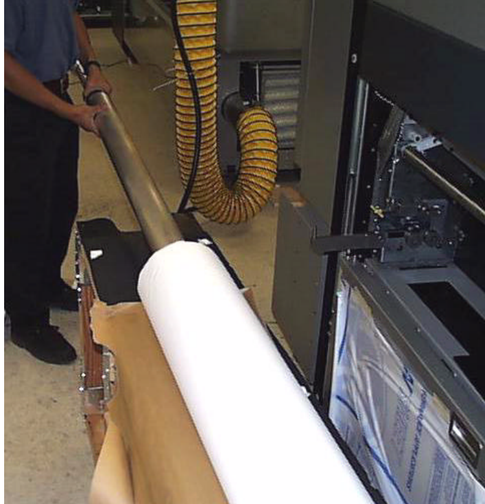
Figure 3-3 Media Support System and Installing Media on the Mandrel
