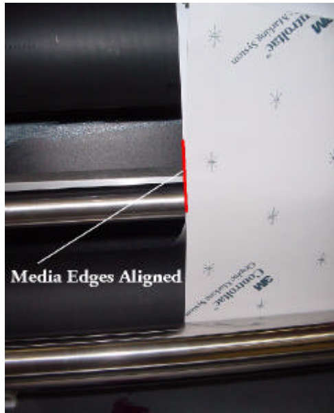
Figure 3-15 Media Edges Aligned
