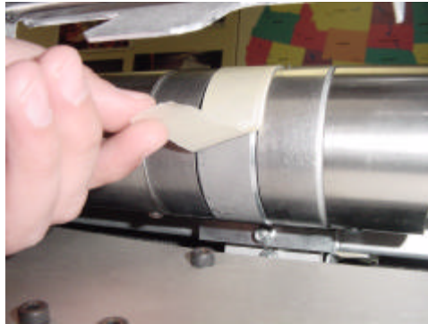
Figure 5-3 Press Fresh Tape on the Encoder Wheel
