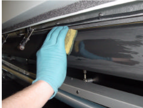
Figure 5-1 Cleaning the Media Drive Roller
