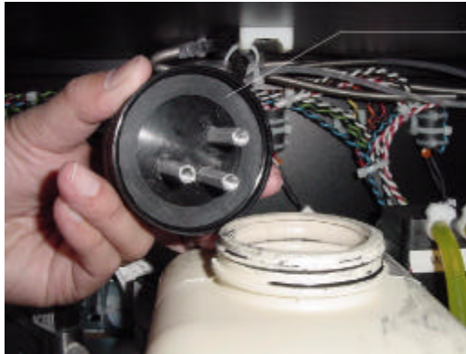
Figure 2-4 Waste Bottle Cap and Gasket
