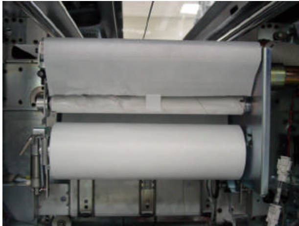
Figure 5-14 Attach the Cloth to the Take-up Core
