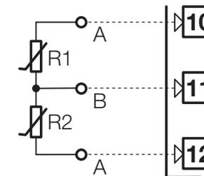
Use wires of the same length and 1.5 mm<sup>2</sup> size.
