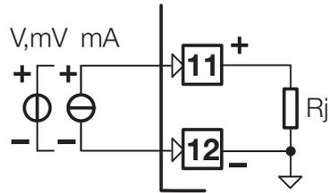
Input resistance =  $30\Omega$  for mA reading;
