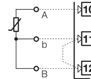
Only for two wires system, put a jumper between terminals 11 and 12.
