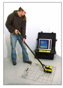
The grid scan mode is used to collect line-scan data in two directions using a specific test grid. The **Conquest<sup>TM</sup>** system comes with plastic and paper sheets on which a 600 x 600 mm (or  $24 \times 24$  in.) test grid has been marked. A single sheet or multiple sheets are taped to the
