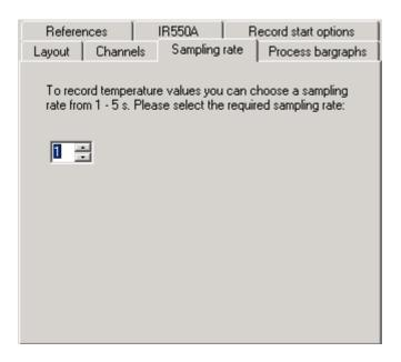
The sampling rate can be set in a range from 1 - 5 s. It defines the equidistant time slices when a new value for recording is requested from the IR 550 A. The default setting is 1 second and should not e modified without need.
