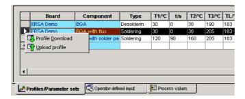
Working with the profile table Upload of profile parameters
