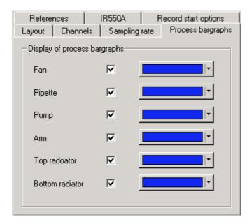
The user can select, which parameter will be displayed and can set the colour of each bar graph line.
