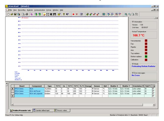
On the top the menu bar is located. Below you will find the toolbars. On the right side the state window is docked. At the bottom of the screen you will find the windows "process values", "operator defined input" and "parameter sets". They are displayed as three functional indices. A more detailed description will be given in the following sections.
