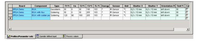
A certain set of parameters can be correlated to a specific application, defined by the board and the component. Moreover it is possible to define a profile to be used for soldering or desoldering a component.
