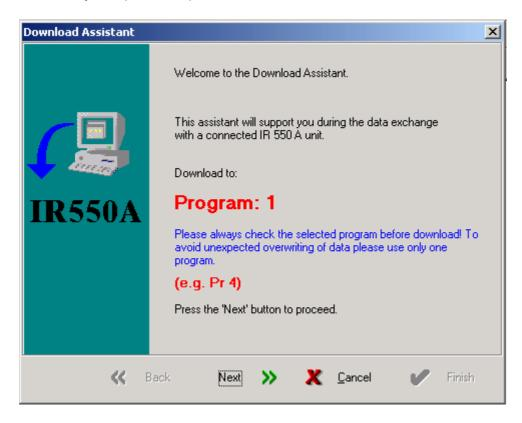
By pressing the 'Next' button all necessary steps will be carried out and checked. In the last view of the assistant you have to press the 'Finish' button and the download will take place.
