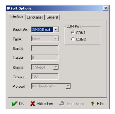
In this dialogue the transmission parameters of the selected COM port are displayed. The user can modify them. The user has the possibility to choose the COM port the null modem cable is connected to and set the baud rate.
