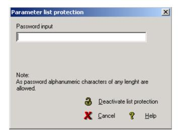
By typing in the correct password and pressing the 'Deactivate list protection' button the protection will be deactivated. The parameter set table can now be changed.
