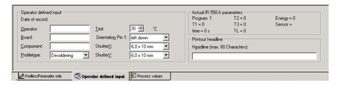
The user is able to edit the actual board and the correlated component, the profile type, the orientation of the component and the shutter settings. On the right side the actual parameters of the selected program of the IR 550 A unit are displayed. This information is automatically updated; changes on the IR unit are possible all the time. In this view the user gets quick information about the units parameter set.
