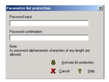
As password the operator can choose any combination of alphanumerical characters. To activate the protection you have to press the 'Activate list protection' button. Now changes on the parameter sets list are not stored.
