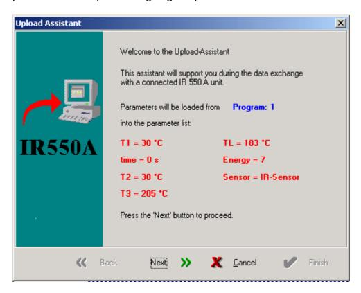
By pressing the 'Next' button all necessary steps will be carried out and checked. In the last view of the assistant you have to press the 'Finish' button and the upload will take place.
