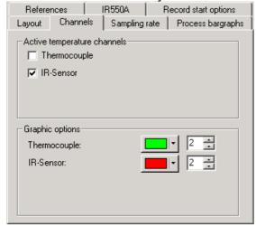
Additionally for the selected channels colours and line sizes can be set.
