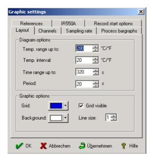
On the Layout index you will find settings for visualisation the temperature profile. The user can set the temperature range and the time range to be displayed. Additionally settings for the grid can be made.
