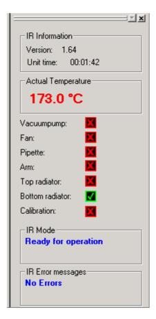
Messages and the display of the actual mode are shown as well as the calibrated temperature from the IR 550 A system (*Depict able channels*).
