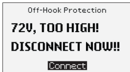
Figure 3-2. Over voltage warning.
