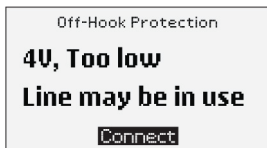
Figure 3-4. Line in use warning.
