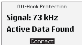
Figure 3-5. Data Present Warning.
