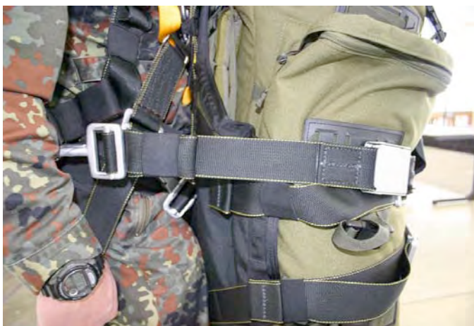
Picture 13 Stabiliser strap connected and tightened.
