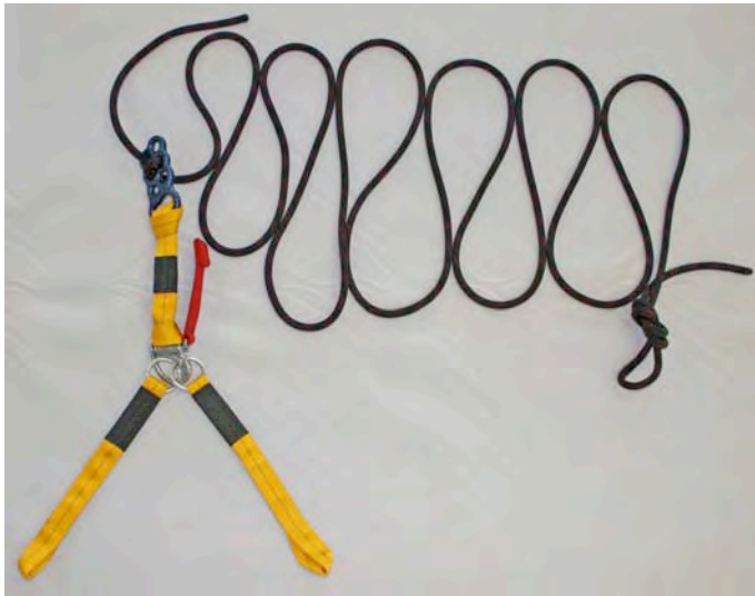
Picture 4 Lowering system with emergency release and lowering line.
