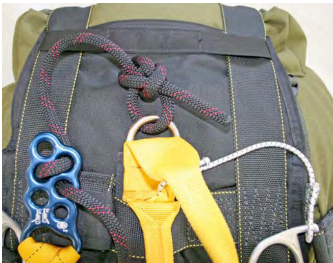
Picture 5 Lowering line connected to the cargo harness.
