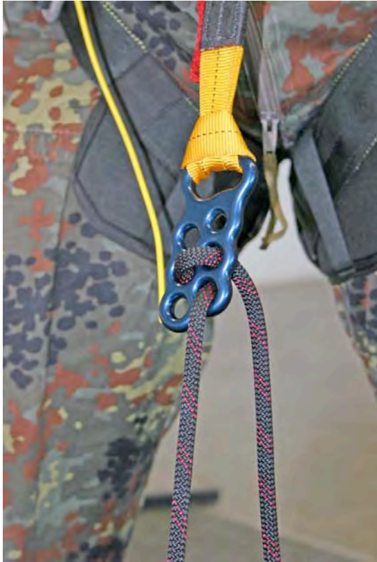
Picture 15: Correct guidance of the lowering line.
