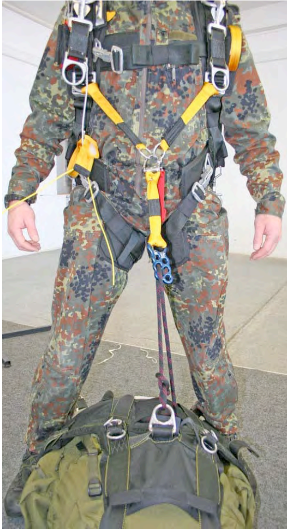
Picture 6 Shows the lowering system attached on a released cargo bundle.
