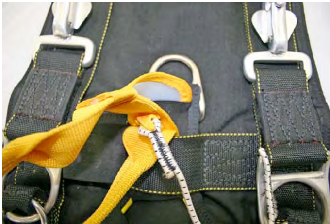
Picture 8 Securing the release handle in it's elastic keeper.
