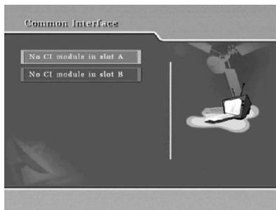
This receiver is equipped with two slots of Common Interface. When a common interface CAM is inserted inside the PCMCIA slot, the receiver detects the type of the CAM automatically and display in the menu.
