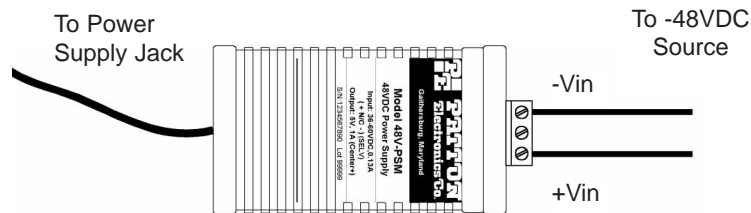
Figure 8. Connecting DC Power to the 48V-PSM DC Power Supply.
