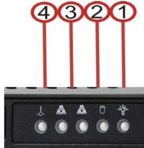
Fig. I-2: QX1000's Front Panel LEDs
