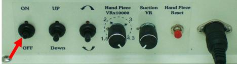
3. Push up or down to adjust working chamber to level the working position.
