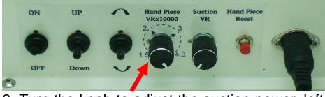
6. Turn the knob to adjust the suction power, left for lower and right for higher
