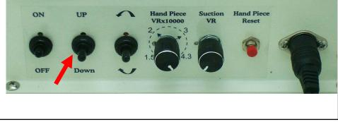
4. Push up or down to select and start the micro motor spin direction CW or CCW.
