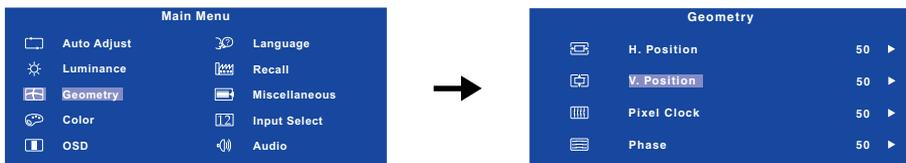
Then, use the ◀ / ▶ Buttons to change the vertical position settings. The vertical position of the overall display should be changing accordingly while you are doing this.
