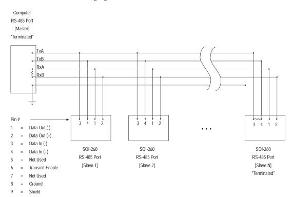
Note: You should terminate the network master computer and the last SOI-260 with a  $120\,\Omega$  resistor. You should also connect the shield wire to ground at the master computer.
