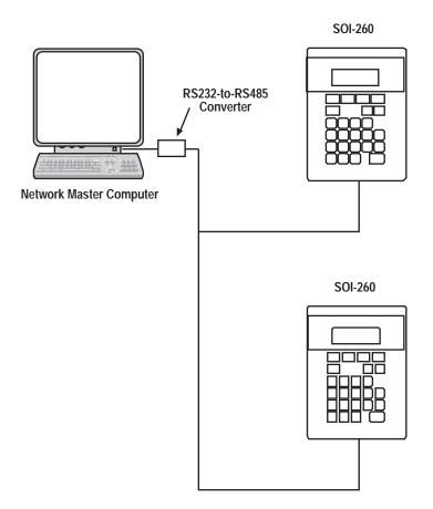
The network master initiates all communications, sends commands (strings of ASCII characters) across the data link, and polls the SOI-260s for responses. To prevent all of the SOI-260s from responding at the same time, each SOI-260 is assigned a unique network address.
