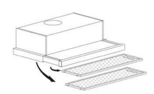
First remove the grille by pulling down on it. Undo the side catches.
