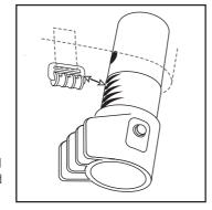
Pryde mast bases already carry this trim zone. When in the correct tuning range, the tack pulley will be as shown.
