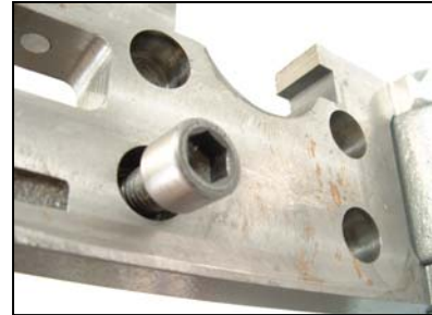
Fig 2. Part 9008 with Counter Bore Holes
