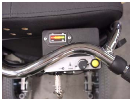
Figure 2 ( Operating panel Kontiki, motor-assisted )
