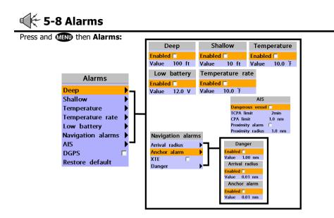
A warning message with beep sound is displayed when an alarm condition is met by user setting. Press (S) to clear the alarm. However, the alarm will be displayed again when the alarm condition occurs again. The unit provides alarms for various functions.
