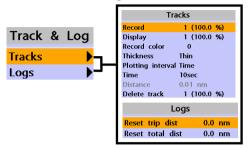
The unit has the capability to store 10 individual tracks and record up to 15,000 track points. Before using the track function you will need to setup the track function that suits your boat.
