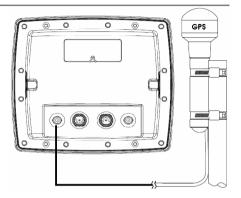
Please check the installation distance between GPS antenna & other equipments. VHF antenna : 3M Compass : 1M
