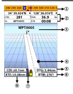
The Highway window shows a 3D view of the vessel traveling through the water when navigating to a destination point.
