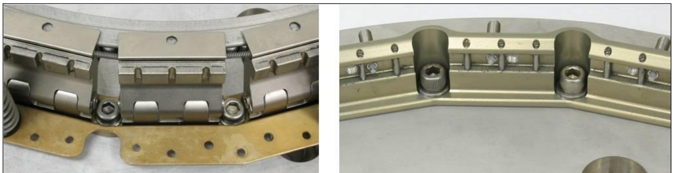
Figure 13: Separated Lightband halves attached to adjoining structures.
