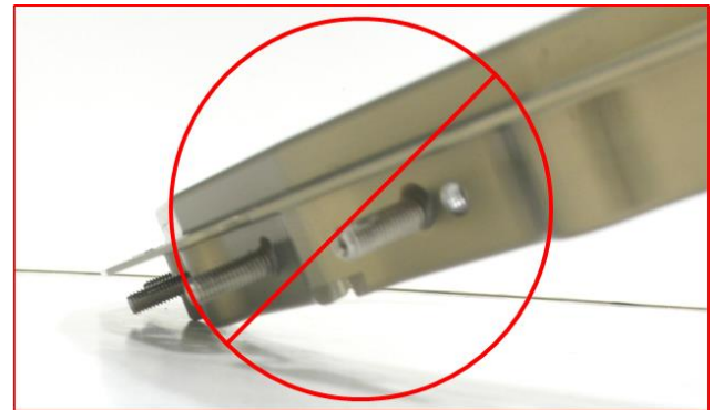
Figure 9: Do NOT touch spring plungers or allow them to contact the table.
