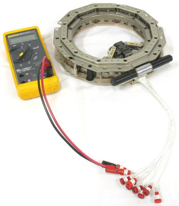
Figure 44: DMM and DB-9 breakout cable used to measure Motor Bracket Assembly resistance.
