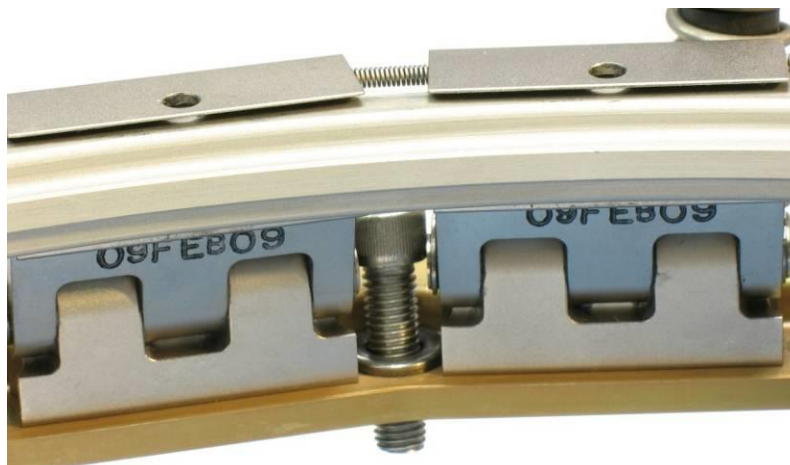
Figure 35: Removing a SHC screw from the Lower Ring, inner view
