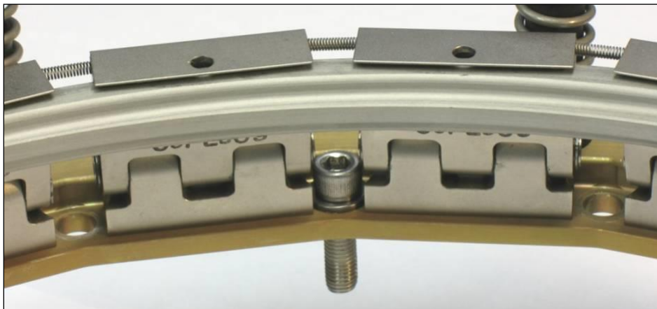
Figure 12: SHC screw and washer inserted between Leaves on elevated Lower Ring.
