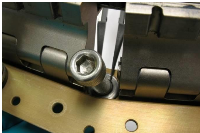
Figure 34: Removing a SHC screw from the Lower Ring, outer view
