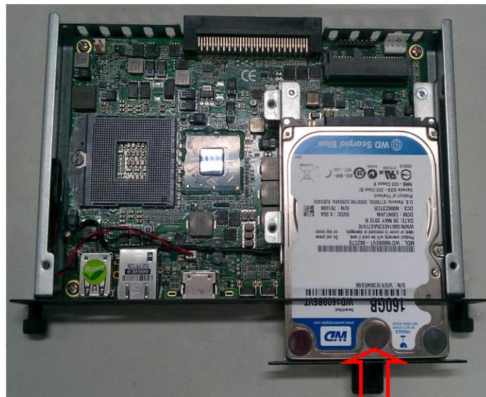
**Step 6.4** Pull the HDD Mylar to slot-out the HDD drive
