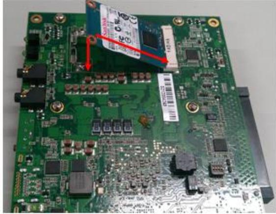
**Step 4.3** Check from right to left on item 3 of SW1 per image illustrated to switch mSATA/mini card function.
