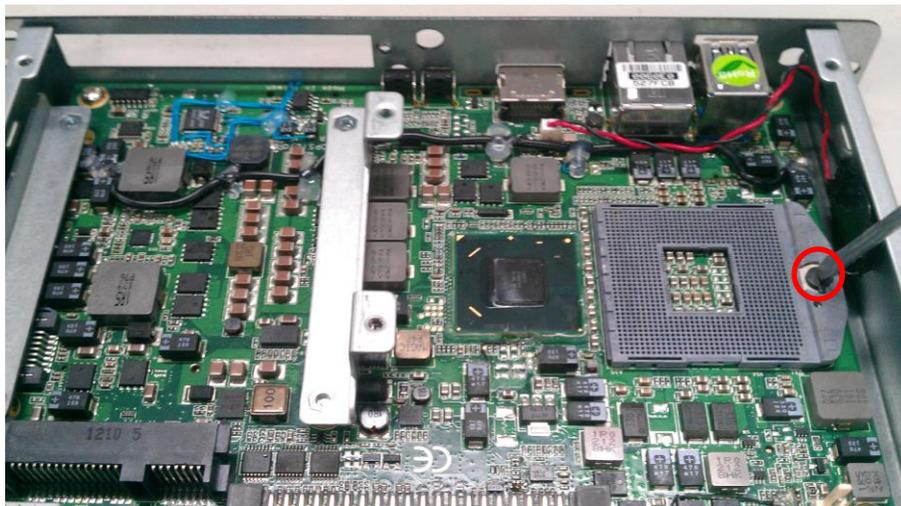
**Step 2.2** Insert the CPU in to the slot. Please follow the indication on CPU as mark and slot to ensure the proper insertion of the CPU
