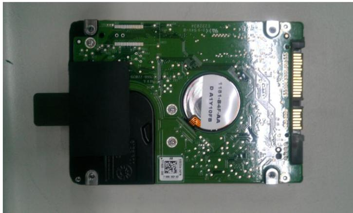
**Step 6.3** Plug HDD drive in to HDD connector
