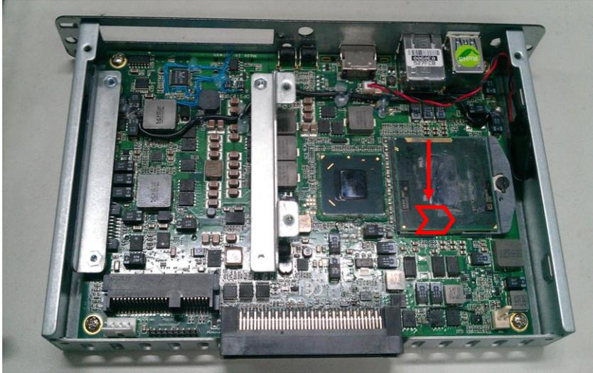
**Step 2.3** CPU is inserted into the socket and the latch is closed.
