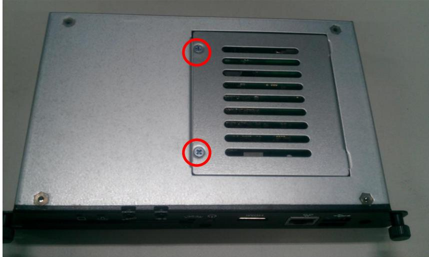
**Step 3.2** After losing the screws, extract the rear of chassis out of the module.
