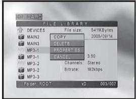
Only support copy files (All data in card or USB device) will copy to CF card. Copy file function can only execute 1 time in each start, to copy for a second time, it would require a restart of the SG If the CF card has insufficient space, the last file copied would be incomplete.
