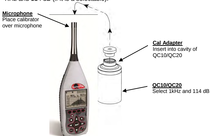
Figure 5-2: Attaching calibrator to SoundPro
