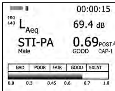
Figure 6-27: Post CAP-1 applied during STI-PA test
