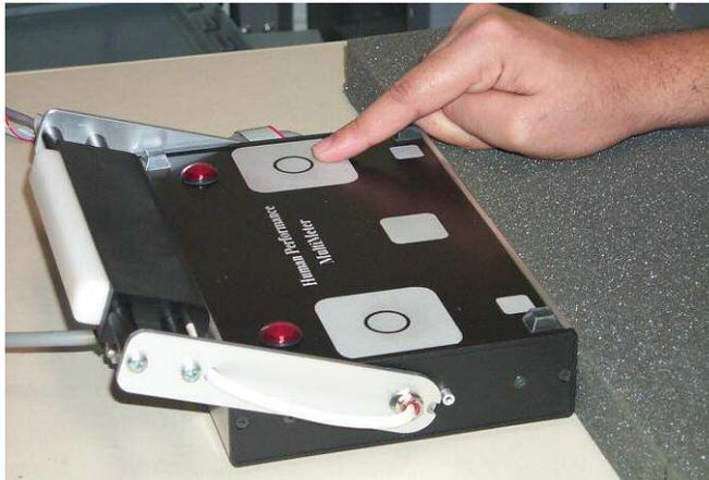
Figure 4.6 Finger Position for Finger Tapping Performance Test.
