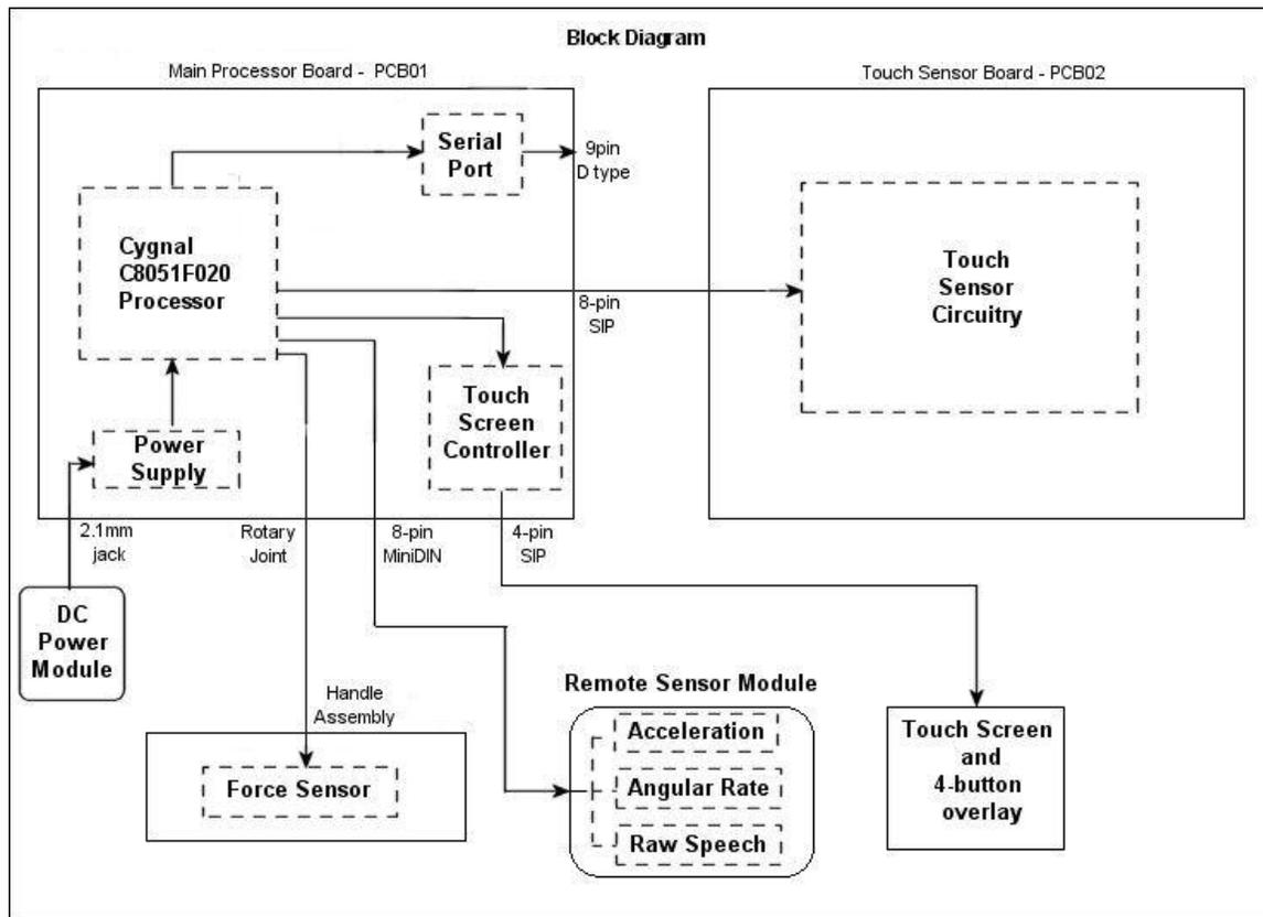
Figure 2.2 HPMM System Block Diagram.
