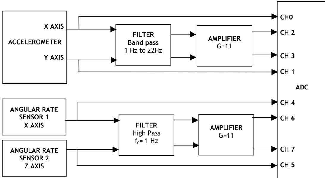
Figure 3.3 Conceptual Block diagram for Acceleration and Angular Rate Subsystems.
