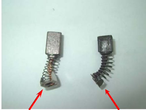
New Motor Brush Worn Motor Brush (Fig 42)
