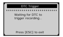
14) Wait for DTC to trigger recording or press ENTER to start recording.
