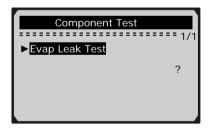
4) If the test has been initiated by the vehicle, a confirmation message will be displayed on the screen.
