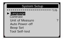
From the Main Menu: Use the UP/DOWN scroll button to select System Setup, and press ENTER button. Follow the instructions to
