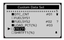
11) Use UP/DOWN scroll button to select a trigger mode and press ENTER button.
