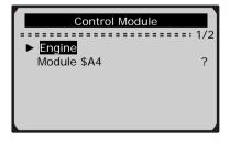
• Use UP/DOWN scroll button to select a module and press ENTER button.
