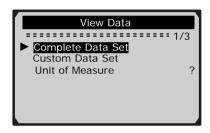
5) View live PIDs on the screen. Use **UP/DOWN** scroll button for more PIDs if an **↑** or **↓** arrow appears on the screen.
