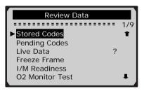
• If no data from previously tested vehicle is recorded, only **Module Present** data containing module ID and protocol type can be reviewed.
