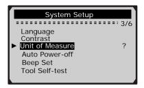
2) From **Unit of Measure** menu, use **UP/DOWN** scroll button to select the desired unit of measurement.
