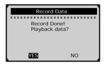
• If you wish to playback recorded data, press ENTER button; if you do not wish to playback, press ESC button, or use LEFT/RIGHT button to select NO and press ENTER button to return to Record Data menu.
