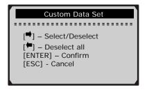
9) Use **RIGHT** button to deselect/select data parameters, and use **UP/DOWN** scroll button to move up and down. Selected parameters are marked with solid squares.
