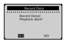
• If you wish to playback recorded data, press ENTER button; if you do not wish to playback, press ECS button, or use LEFT/RIGHT button to select NO and press ENTER button to return to Record Data menu.
