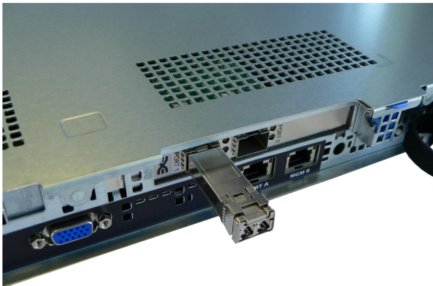
Rear Panel of the Node Showing FC Cable Connections
