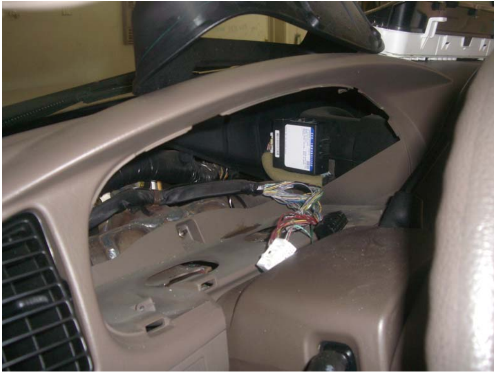
2003 and later Sequoia (34010) immobilizer location behind instrument cluster.
