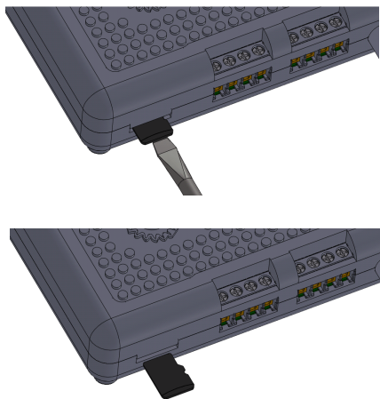
Figure 1.4: Insert microSD card in microSD card slot, use a flathead screwdriver for assistance. DO NOT let the microSD card slide above the slot and fall into the enclosure.
