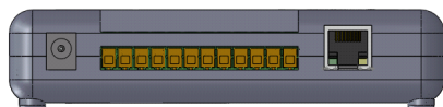
Figure 1.2: Left to Right: DC Power Connector, six output pairs (left positive, right negative), Ethernet connector.
