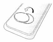
2. Insert batteries matching the + and - signals. (Battery Type: CR-2025)
