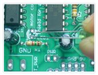
Next is the 3mm LED used to indicate motor power. LEDs are polarized, just like capacitors, and the long lead is the positive (+) lead.
