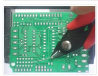
Clip the long leads, just above the solder joint using diagonal cutters.
