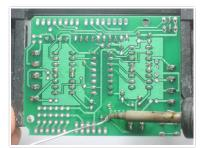
Solder in the 3 pieces of header and the three terminal blocks.
