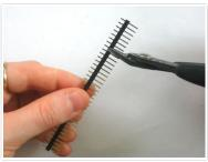
Next its time to make the headers for the jumper, servos and arduino.
