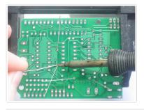
Using your soldering iron tip, heat the resistor wire lead and the metal ring (pad) at the same time, after a few seconds, poke a little solder in so that it melts into a nice cone. Remove the solder and then remove the solder and then remove the soldering iron. Do this for all 4 wires.
