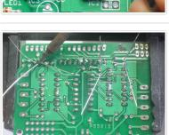
After double-checking their polarity, solder and clip the three capacitors.
