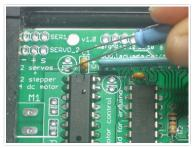
Next are the three 100uF electrolytic capacitors C1, C3and C5. Electrolytic capacitors are polarized and must be placed in the correct orientation or they could pop! The long leg of the capacitor is the positive (+) leg and goes into the hole marked with a +. The close-up images shown here indicate with hole is the + one.
