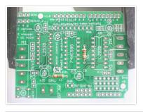
Next, slip the resistors into the PCB as shown, so that they sit flat against the circuit board. Bend the wire legs out a bit so that when the board is flipped over
