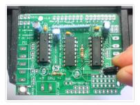
Place the two 47uF remaining electrolytic capacitors, **C7** and **C8**
