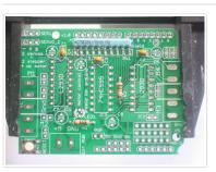
Next is the 6mm tactile switchRESET and the resistor networkRN1. The tact switch is used to reset the Arduino since its not possible to reach the reset button once the motor shield is on.
