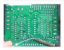
Flip the board over and solder in the resistor network and switch. You won't need to clip the leads as they are quite short aleady.
