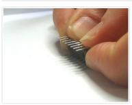
Next are the three integrated circuits (ICs) IC1, IC2 and IC3. When ICs come from the factory, the legs are angled out somewhat which makes it difficult to insert them into the PCB. Prepare them for soldering by gently bending the legs against a flat tabletop so that they are perfectly straight.
