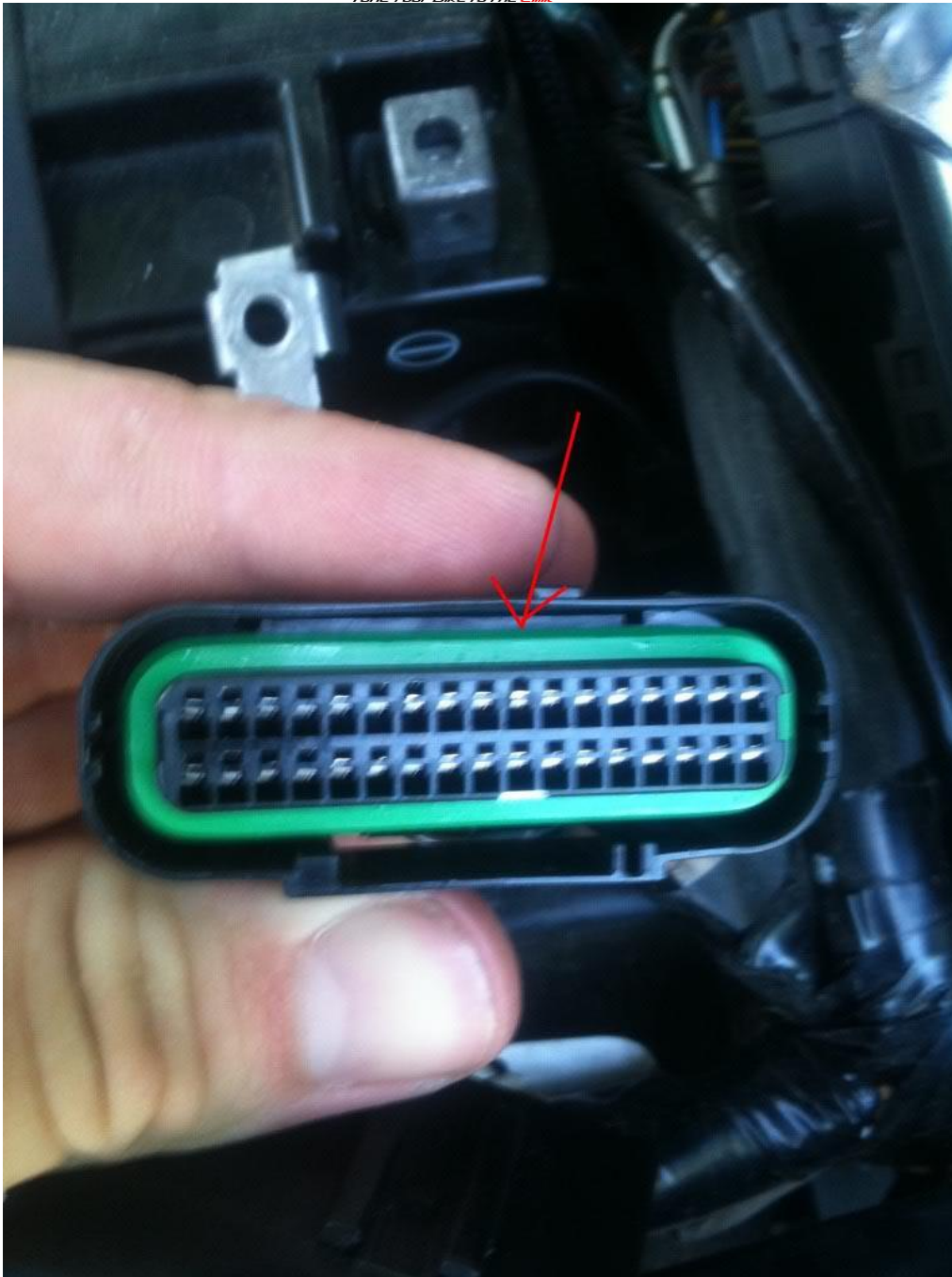
View of ECU plug with 2 wire harness installed
