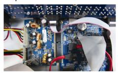
**Note:** Please make sure the power cable of the DVD writer is plugged into the black jack. This power jack can supplied power to one hard disk and one DVD writer simultaneously.
