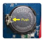
Step5: Get a new battery with the side of "CR2032" facing up, and install it to the mainboard.
