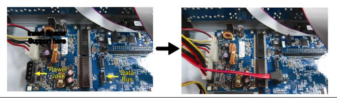
**Note:** Please make sure the power cable of the DVD writer is plugged into the black jack. This power jack can supplied power to one hard disk and one DVD writer simultaneously. The white jack is used to supply power to only one hard disk.
