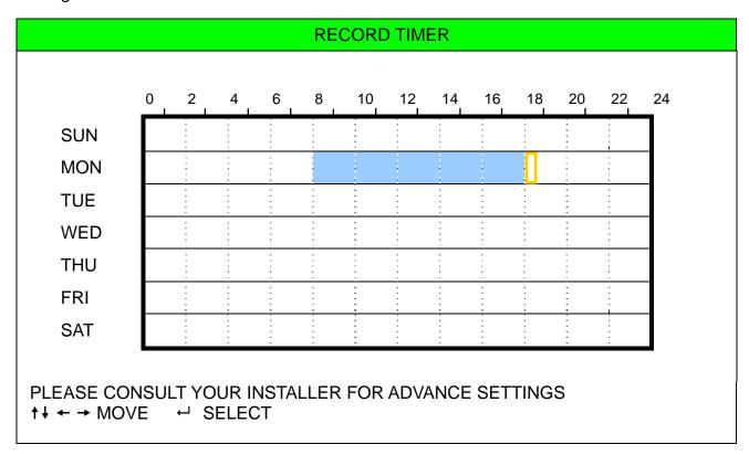
**X axis**  $0 \sim 24$  hours. Each time interval within a square is two hours (divided into four 30-minutes).
