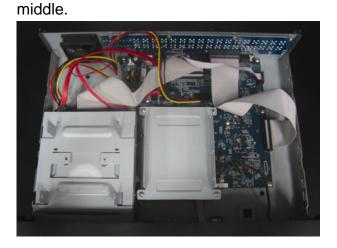
STEP2: Install the compatible HDD to the bracket.
