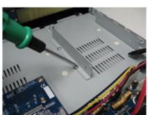
b) Get a compatible SATA HDD, and connect it to the power connector and data bus connector.
