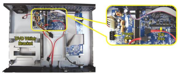
Step2: Put the DVD writer in the bracket, and fix it to the bracket with two screws on each side.
