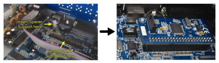
Step6: Connect the data bus and power cables to the data bus and power jack on the DVR main board as illustrated below.
