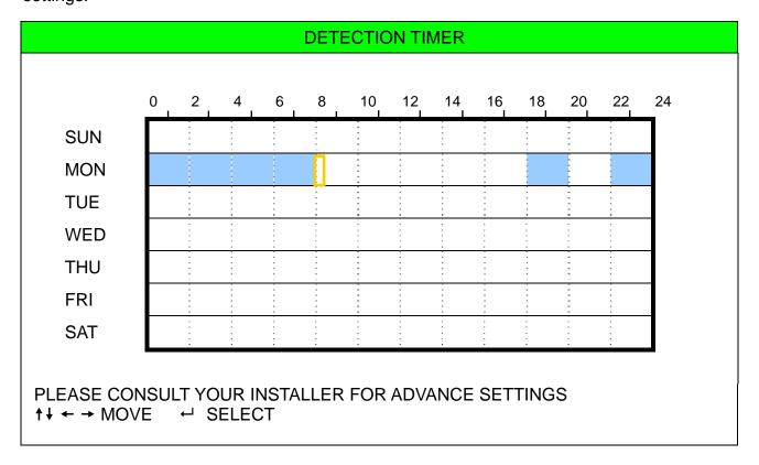
**X axis** 0 ~ 24 hours. Each time interval within a square is two hours (divided into four 30-minutes).
