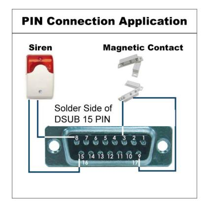
**Siren:** When the DVR is triggered by alarm or motion, the COM connects with NO and the siren with strobe starts wailing and flashing.
