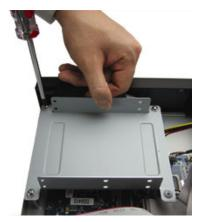
b) Get a compatible SATA HDD. Slide the HDD to the bracket, and fix it with two screws for each side. There are three screw holes per side on the bracket, and you can choose two of them to secure the HDD.
