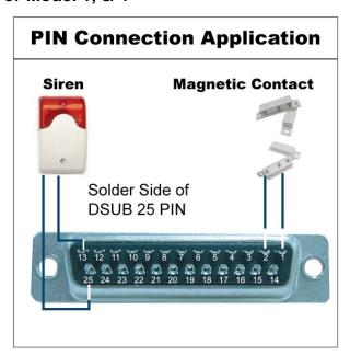
**Siren:** When the DVR is triggered by alarm or motion, the COM connects with NO and the siren with strobe starts wailing and flashing.
