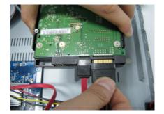
c) Put the HDD to the DVR, and have the SATA HDD fixed in the DVR.
