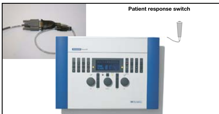
Fig. 11 USB/RS232 connection for PC or Laptop with USB port or RS232 cable for PC or Laptop with serial port
