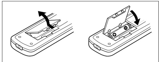
Open the lid of the battery compartment on the rear of the remote control unit, and insert the batteries, taking care to align the ⊕ and ⊖ polarities correctly.
