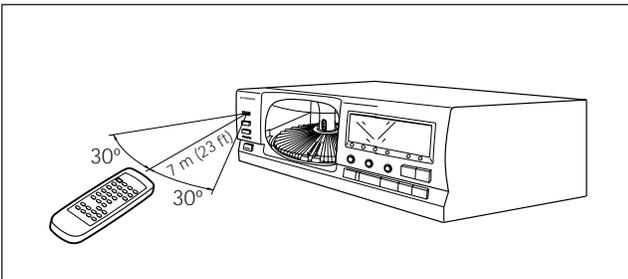
When operating the remote control unit, point the unit's infrared signal transmitter at the remote control receiver (Remote Sensor) on the front panel of the player. The remote control unit can be used within a range of about 7 meters (23 feet) from the remote sensor, and within angles of up to about 30 degrees.
