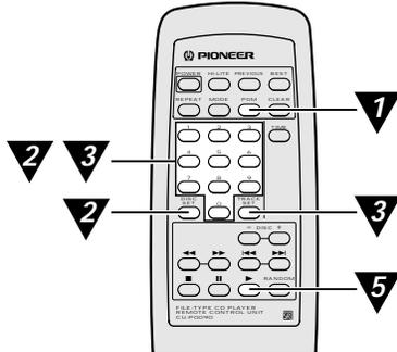
Operation example: Programming disc 2, track 7 as step 1, and disc 5, track 3 as step 2.
