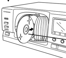
Loading the disc into the Single Loader slot with the label side (printed surface) facing to the left.
