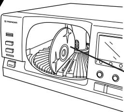
Load the disc into the rack with the label side (printed surface) facing to the left.
