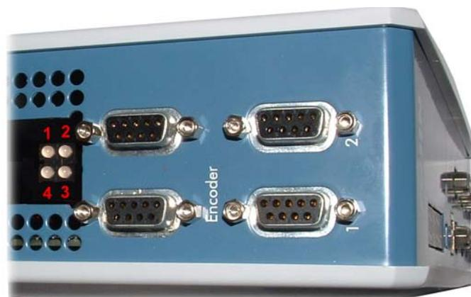
**Figure 3. AnyBus Status LEDs numbering**
