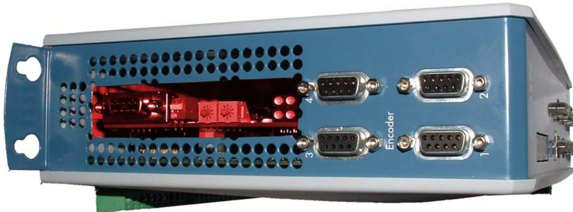
**Figure 1. Photograph of AnyBus interface on QManager/QControl4**
