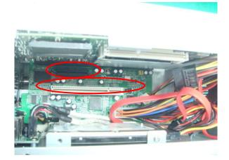
**Step 5** Align the PCI or PCIe card with the slot, and press the card into the slot until it is firmly seated.
