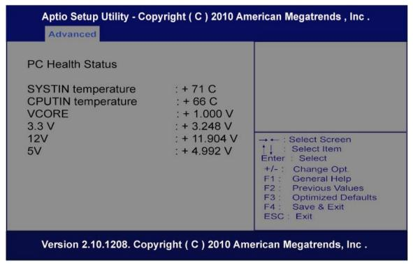
This screen displays the temperature of system and CPU, cooling fan speed in RPM and system voltages (VCORE, +12V, +5V and +3.3V).
