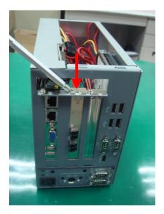
**Step 6** Close the top cover back to the chassis and fasten all screws.
