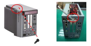
**Step 4** Locate the PCI or PCIe slots from the side.
