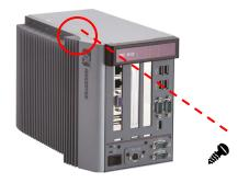
**Step 4** Open the top cover and locate the two Hard Disk Drives from the side.
