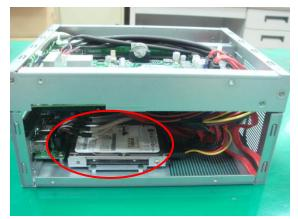
**Step 5** Use assembly parts to fix HDD with the bracket.
