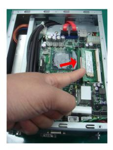
2. Install the memory module into the socket and push it firmly down until it is fully seated. The socket latches are clipped on to the edges of the SO-DIMM.
