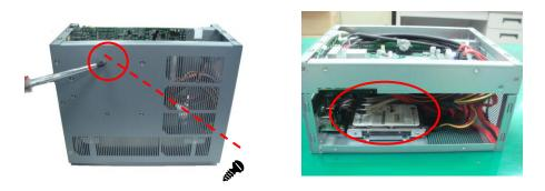
**Step 7** Close the top cover back to the chassis and fasten all screws.
