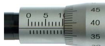
Figure A3.2 Example 1: reading = 10380\ \mu\text{m}
