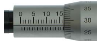
Figure A3.3 Example 2: reading = 16780 \mu\text{m}
