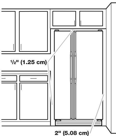
To ensure proper ventilation for your refrigerator, allow for 1/2" (1.25 cm) space on each side and at the top. When installing your refrigerator next to a fixed wall, leave 2" (5.08 cm) minimum on each side (depending on your model) to allow for the door to swing open. If your refrigerator has an ice maker, allow extra space at the back for the water line connections.
