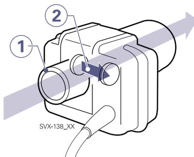
1. Gas flow through the airway adapter in the capnostat sensor.
