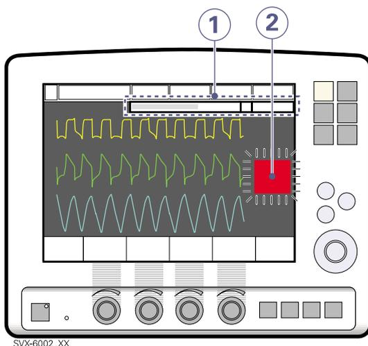
When an alarm is activated, the following information is supplied on the screen.
