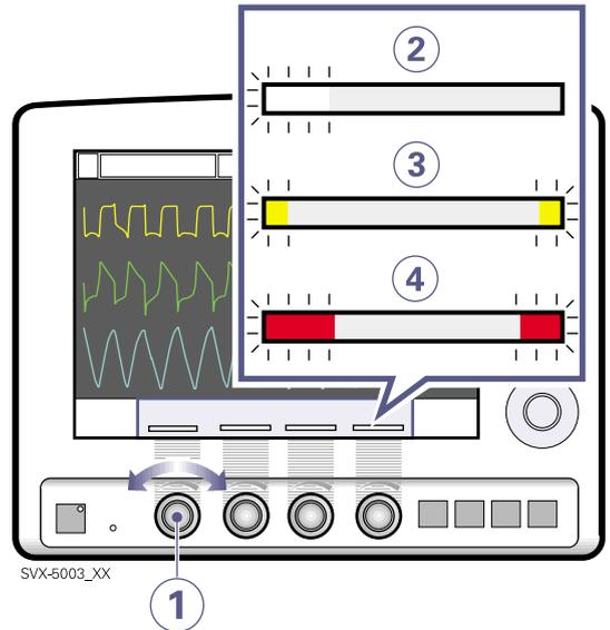
The four Direct Access Knob parameters are displayed at the bottom of the screen with color-coded bars that indicate whether the parameter values are within generally-recognized safety limits.
