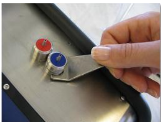
PICTURE 37. Loosen the inlet by using the spanner.
