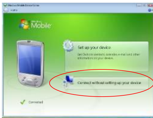
PICTURE 106. Initial connection screen. Press “Connect without setting up your device”.
