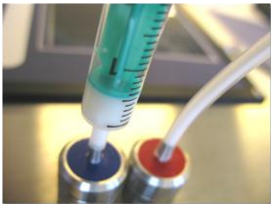
PICTURE 29. Leave the syringe on the inlet during measurement and check.
