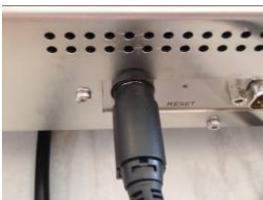
PICTURE 13. Correctly attached power plug.
