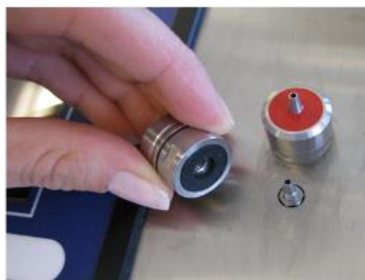
PICTURE 38. Remove the inlet.
