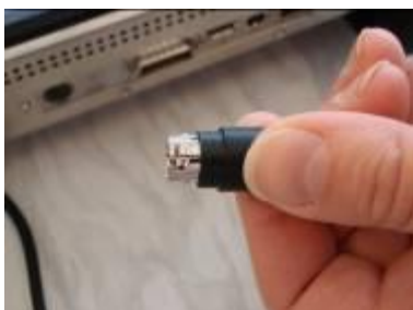
PICTURE 9 and 10. Pull back the plastic cover.
