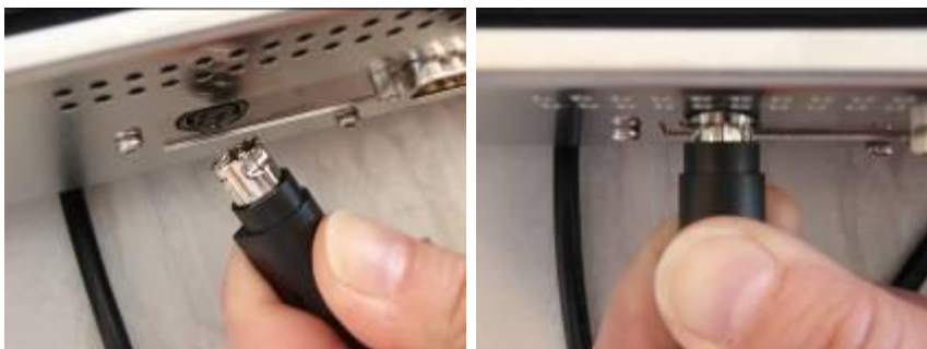
PICTURE 11 and 12. Keep the cover pulled back and insert the plug.
