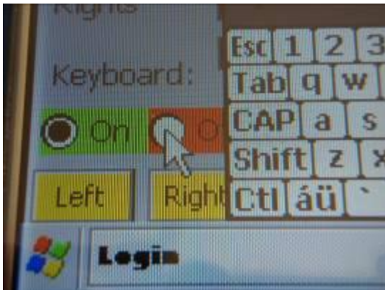
PICTURE 18. Detailed description of where to turn the keyboard on and off.
