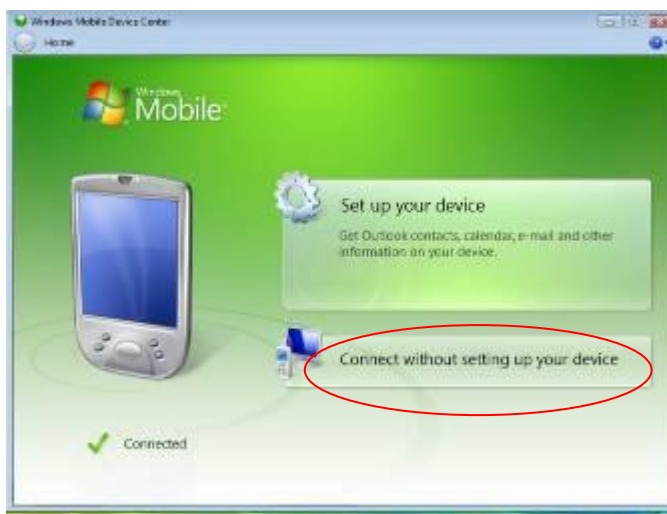
PICTURE 66. Initial connection screen. Press “Connect without setting up your device”
