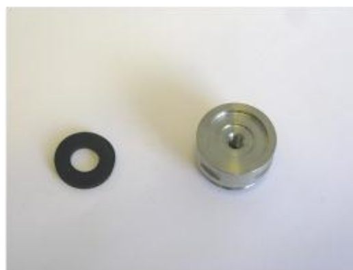
PICTURE 40. Gasket removal.
