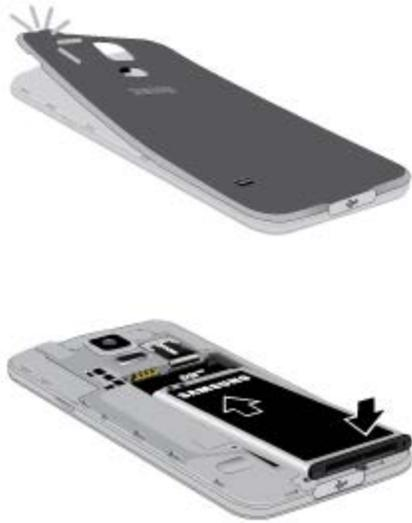
**Important:** Before closing the cover, check to see if there is any foreign substance such as dust or sand between the rubber on the back of the cover and the sealing area.
