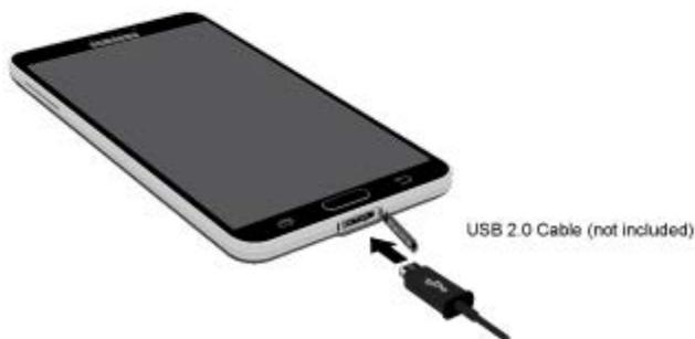
**Note:** Your phone supports USB 3.0 and USB 2.0, and includes a USB 3.0 cable for higher data transfer speeds when connected to another USB 3.0 device. You can also use USB 2.0 cables (not included) to charge and connect your phone.
