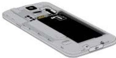
1. Using the slot provided, gently lift the cover off the phone.
