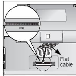
• Connect the flat cable into the optional connector on the keyset, making sure that it is connected securely.
