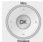
Sometimes a system does not show all message for some operation, then the arrow key will be displayed the begin or end line. By pressing a navigation key of LDP-7000 series, others will be displayed.
