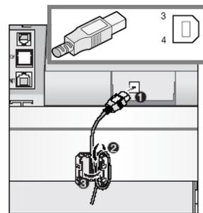
• When connecting the USB cable to USB, a ferrite core must be attached for suppressing EMI. (Wrap the cable once around the ferrite core, then close the case of the ferrite core. Attach the ferrite core 3 cm away from the connector.)
