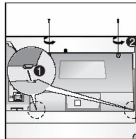
• Hook the option module cover onto the Keyset base (line up the protrusions on the cover with the receptacles on the keyset base). And then turn the screw clockwise to tighten.
