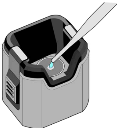
Figure 5. Using a Pipette to Place a Drop of Liquid on the Sample Platform
