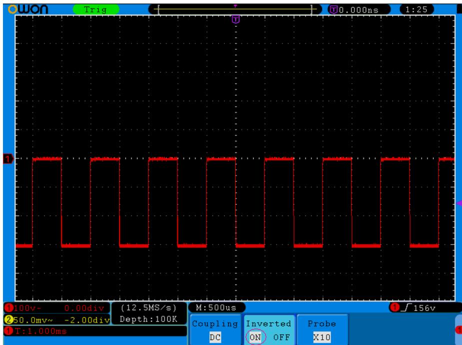
Fig. 5-5 Inverted Waveform
