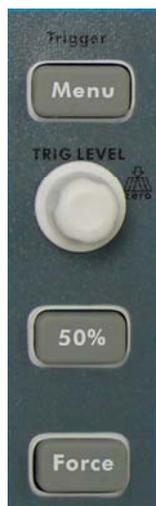
**Fig.4-14** Trigger Control Zone
