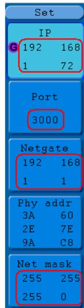
**Fig.5-52** Set the network parameters of the oscilloscope
