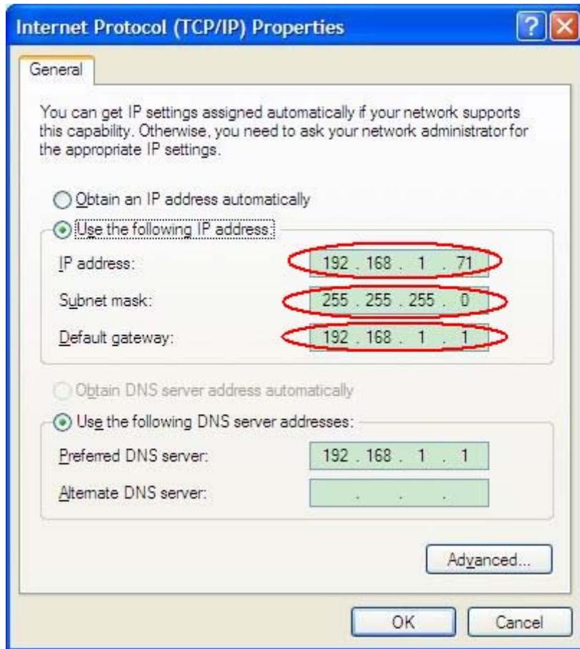
Fig.5-50 Set the network parameters of the computer
