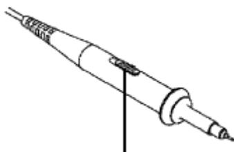
**Fig.4-10** Attenuation Switch
