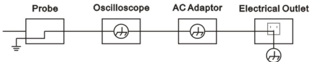
It is not allowed to measure AC power when charging the oscilloscope with adapter.
