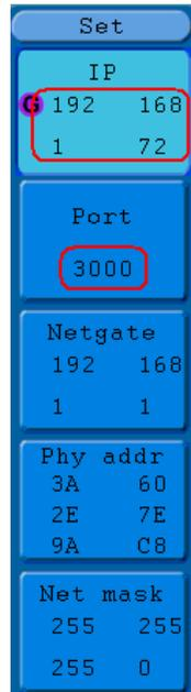
**Fig.5-49** Set the network parameters of the oscilloscope
