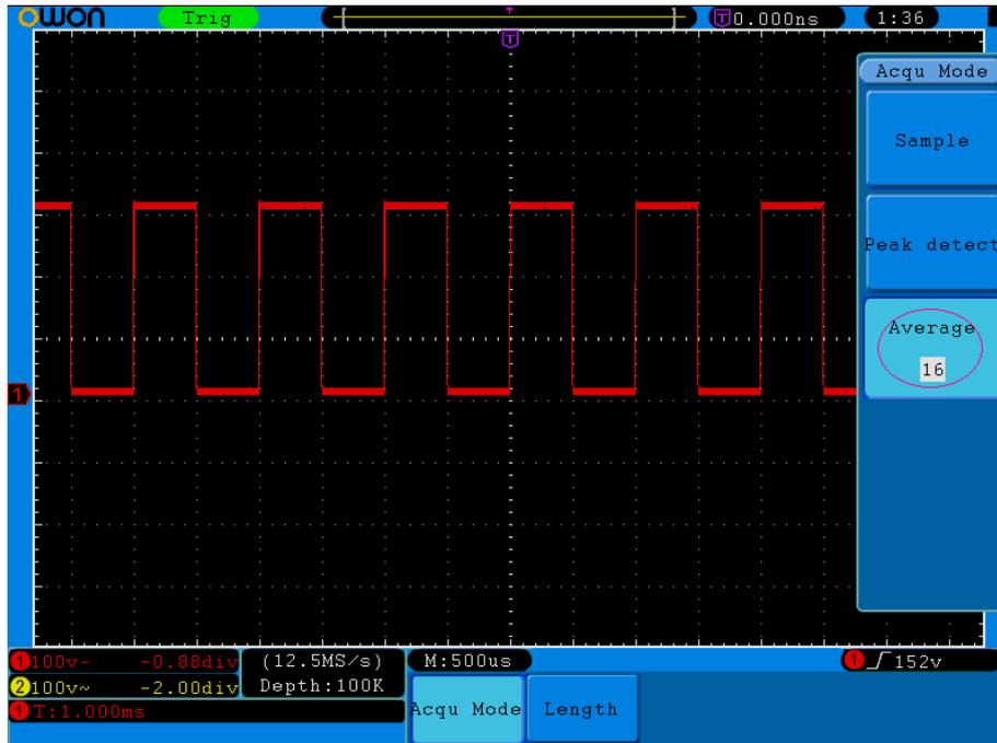
**Fig.6-5** Reduce Noise level by using Average function
