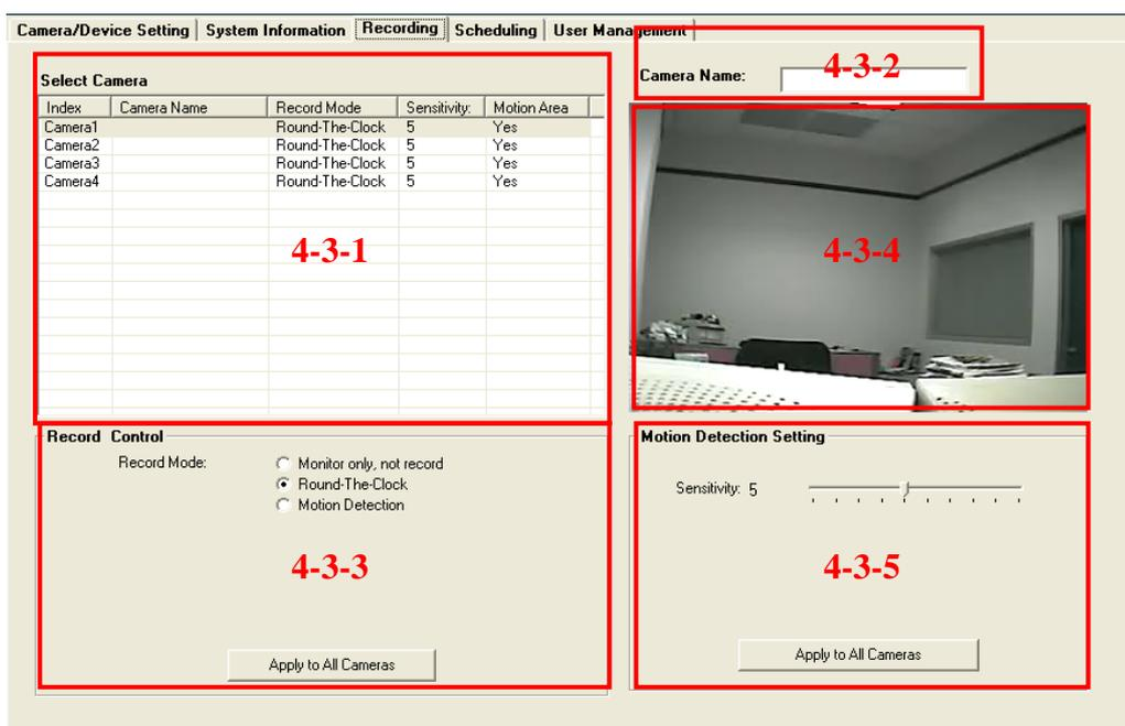
4-3-1 Select Camera: Select a camera and its real-time image will be shown on the right below the camera name.
