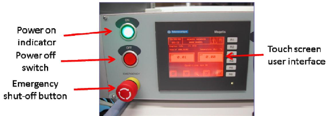
Figure 11 : Left side of control unit front panel, with components marked.
