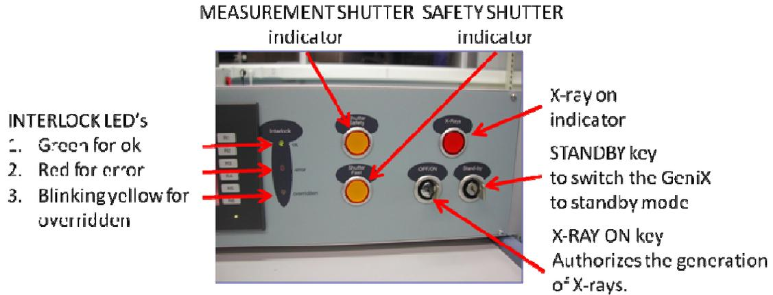
**Figure 12 :** Right side of control unit front panel, with components marked. Note that for the two keys, vertical is off, horizontal is on.
