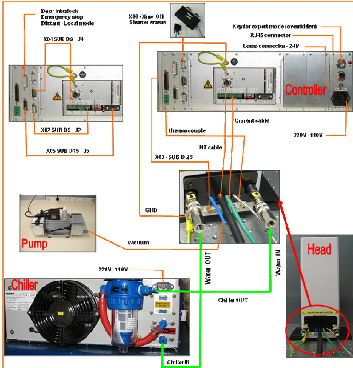
**FIGURE 20 :** Diagram showing the connections for the various GeniX units (optical head, control unit, chiller, and vacuum pump).
