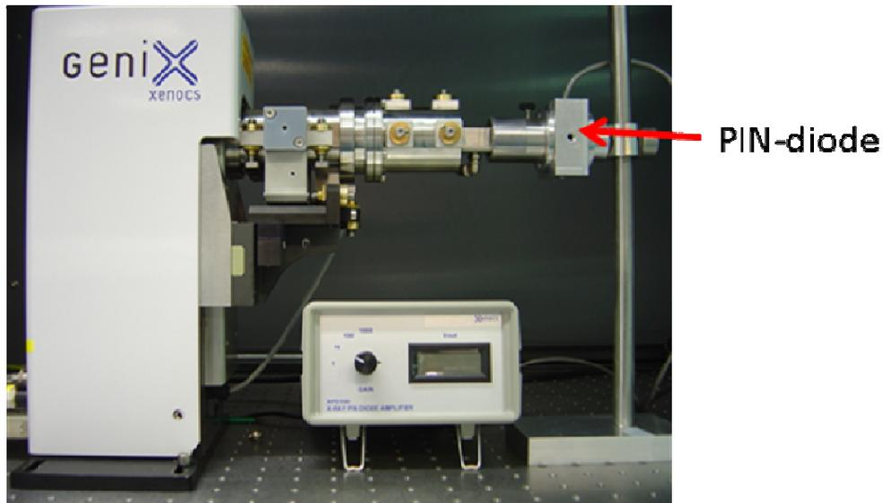
**FIGURE 23 :** View of GeniX optical head with PIN-diode positioned to monitor the beam.
