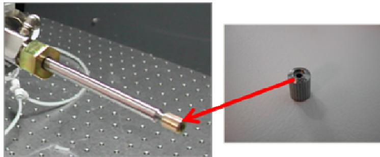
**FIGURE 29** : View of the collimator tube and the pinhole mount.
