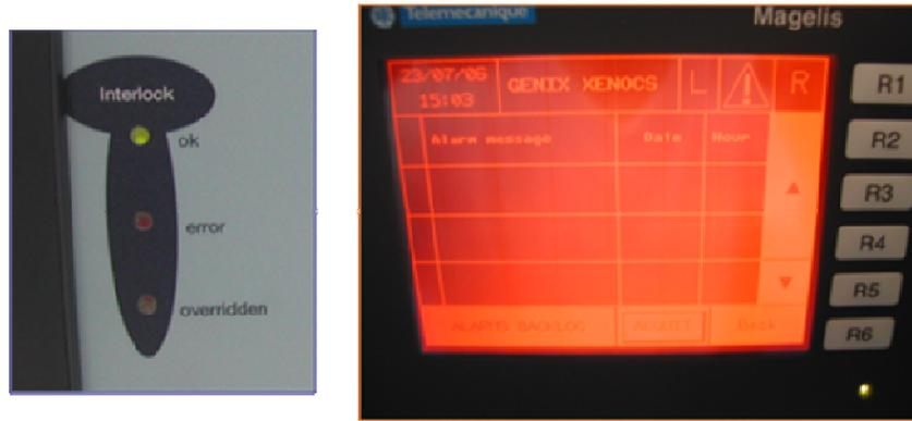
**Figure 17 :** View of interlock LED and interlock screen after interlocks have been closed and “ACQUIT” button pressed. Note interlock screen color is orange instead of red, indicating that all interlocks are closed.
