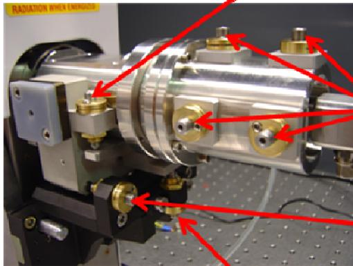
**4 alignment screws for collimator
