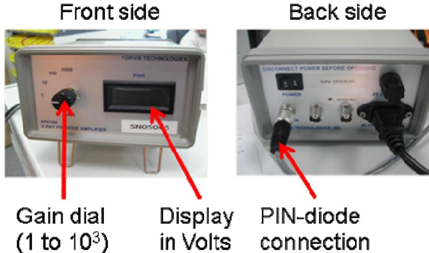
**FIGURE 24 :** View of front and back of PIN-diode.
