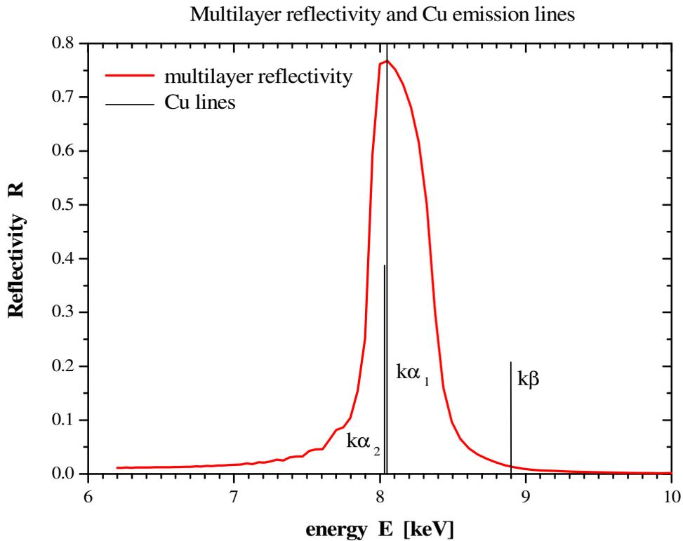
**Figure 5 :** Typical reflectivity curve of a W/Si multilayer optic designed to match Cu  $K_{\alpha}$  emission lines.
