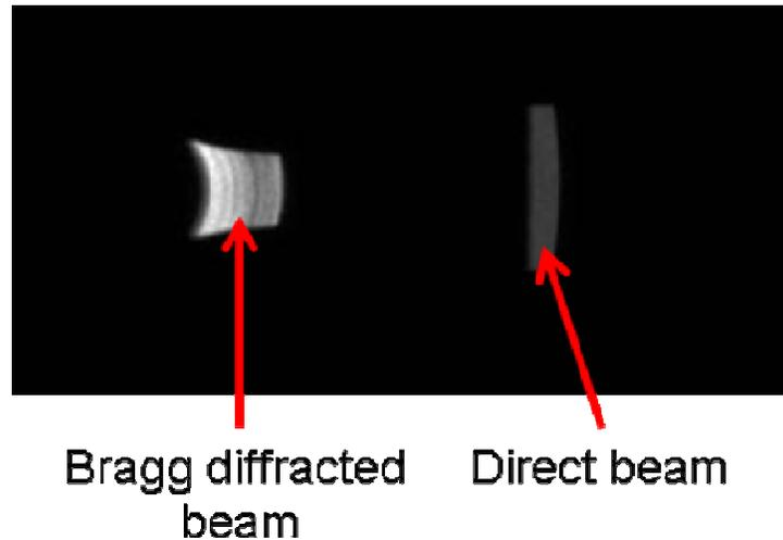
**FIGURE 28** : Image of diffracted and direct X-ray beams.
