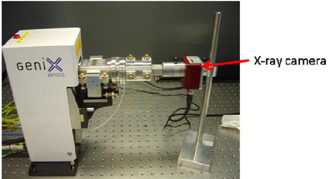
**FIGURE 22 :** View of GeniX optical head with X-ray camera positioned to monitor beam.
