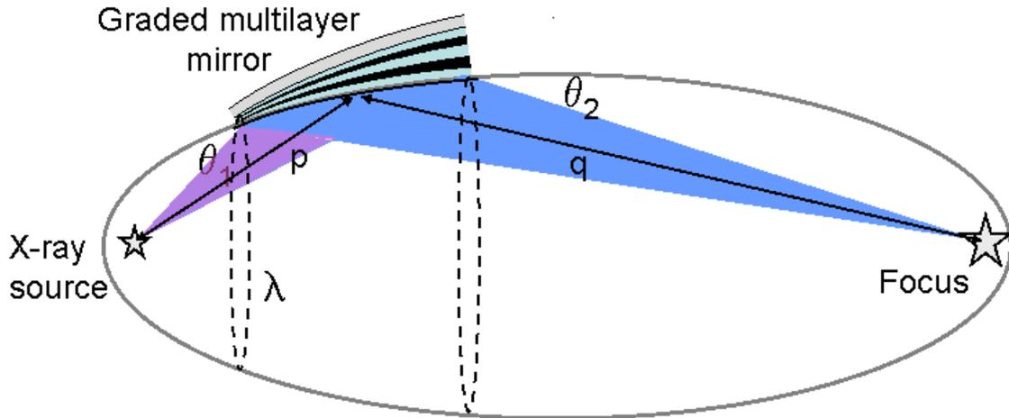
**Figure 6 :** Ellipsoidal mirror with lengths  $p$  and  $q$  indicated. This schematic represents the focusing case. For a collimating mirror with  $q = \infty$  we would get a parallel beam, and the ellipsoid of revolution would be a paraboloid of revolution.
