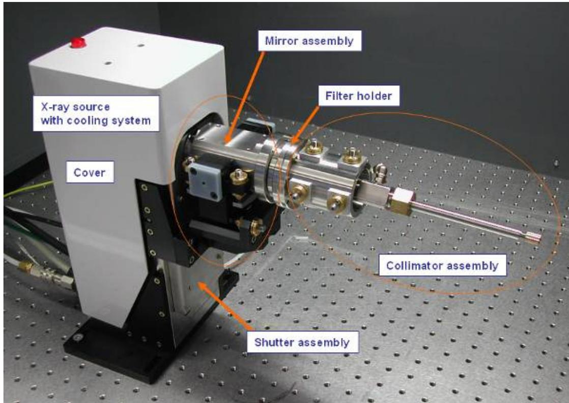
Figure 19 : View of GeniX optical head.
