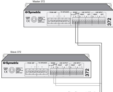
Connect a cable from TRIGGER and Ground terminals of the master unit.
