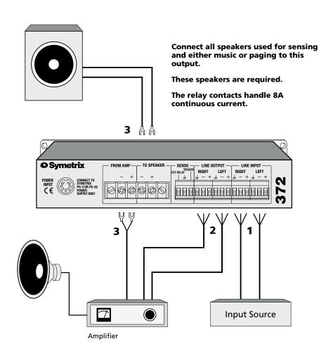
Connect all speakers that do not sense to the amplifier output.
